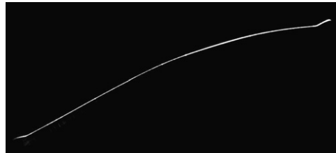
Fig. 2. Membrane shape as obtained from the laser sheet visualization, U_\infty = 5 m/s, \alpha = 20^\circ .
